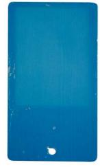
Select 1000 QUV results. Test panel shows less color loss than national brand tested.
